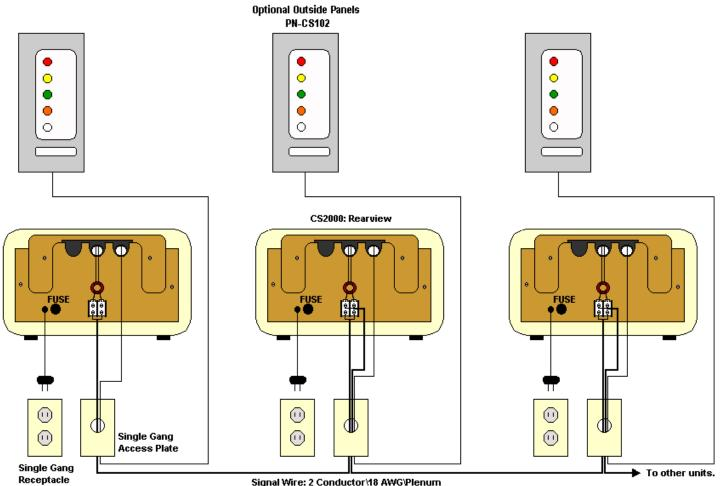
Signal Wire: 2 Conductor/18 AWG/Plenum
